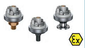
Factory-set pressure switches monitoring overpressure from 5 mbar to 12 bar or vacuum from -5 to -900 mbar of liquid and gaseous – also aggressive – media. Pressure setting and switching differential are individually factory-set.
