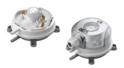
Adjustable differential in IP54 and IP65 pressure switch for monitoring overpressure, vacuum and differential pressure. The medium may be air or other non-combustible and non-aggressive gases.
