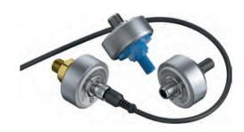
Analogue pressure transmitter monitoring overpressure from 0 to 300 mbar or vacuum from -100 to 0 mbar of liquid and gaseous – also aggressive – media.
