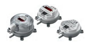
This differential pressure transmitter in IP54 provides up to 8 pressure ranges and 2 analogue output signals, wich are easily slectable on site. Versions with manual or automatic zero point adjustment as well as with or without LED display are available.
